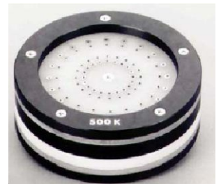
Surface Resistance Calibration Test Fixture
