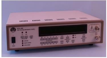
The Trek Model 668B is a precision, high-voltage, reference power supply with an adjustable output voltage range of 0 to 3 kV DC or 0 to -3 kV DC and an output current capability of up to  $\pm 5 \text{ mA DC}$ .
